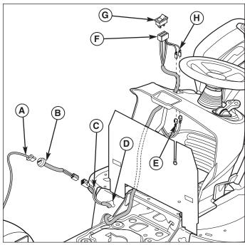
Figure 15. Install Power Port & Switch
